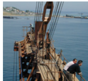
Picture 3.29: Monogirder boom with trolley running at bottom.
