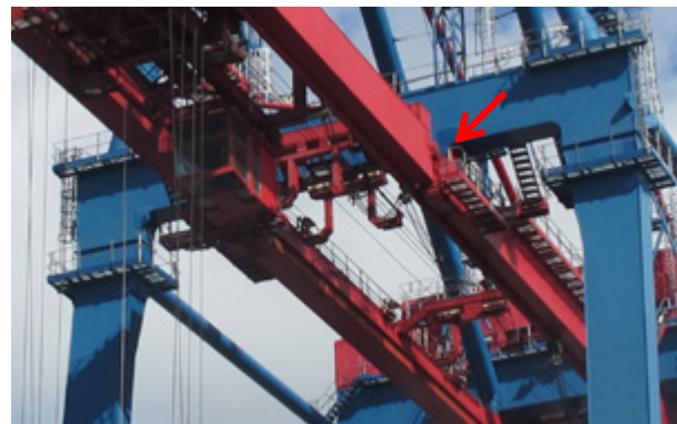
Picture 3.18: WS TGSB of twin girder crane. The arrow points to a detail similar to that shown in 3.17.
