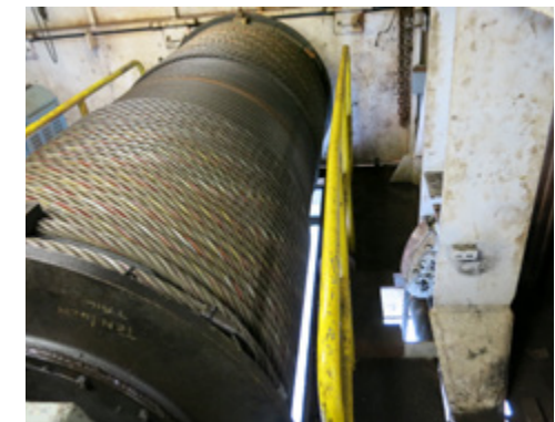
Picture 3.70: Machinery trolley hoist drum on left and rope direction change and dead end on right.
