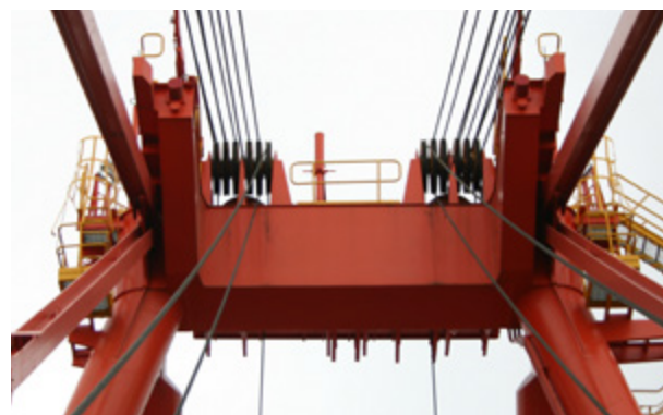
Picture 3.59: Apex beam seen from waterside with forestays on the outside and boom hoist in centre.
