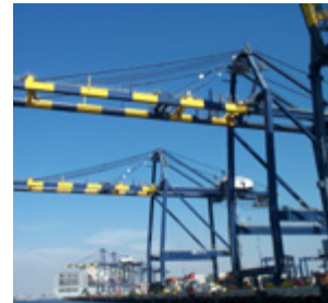
Picture 3.30: Twin girder booms with minimal cross bracing.
