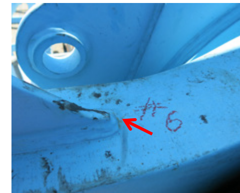
Picture 3.55: A crack indication at the end of a lifting lug on an intermediate forestay link plate.
