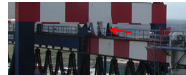
Picture 3.20: WS TGSB of a monogirder crane with pinned connection.
