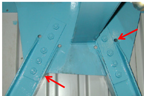
Picture 3.65: Trolley members with likely crack locations indicated.
