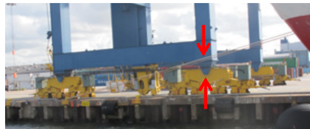
Picture 3.6: Sill beam with legs centered on equalizer pins.
