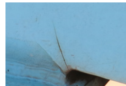
Picture 3.53: A crack at a forestay end connection plate.
