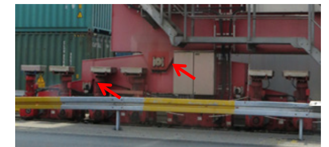
Picture 3.4: RTG crane with 1 wheel per corner.
