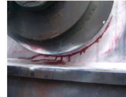
Picture 3.54: A crack at the boss weld on the boom forestay connection plate.
