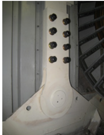
Picture 3.64: Pinned joint at center of trolley frame to allow flexibility and reduce secondary bending due to warping of frame during operation.
