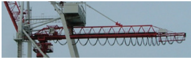
Picture 3.27: Truss type trolley girder.
