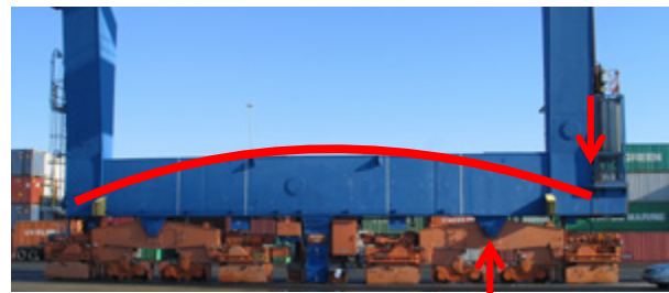
Picture 3.7: Sill beam with legs cantilevered beyond equalizer pins.
