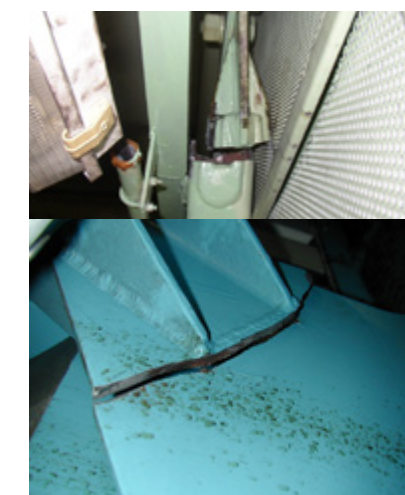
Pictures 2.2 and 2.3: Fatigue fractures of diagonal members on machinery trolleys.
