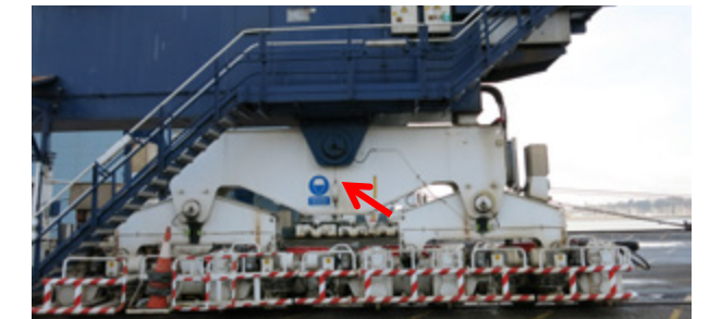
Picture 3.2: STS crane gantry system with 4 of 8 wheels driven per corner.
