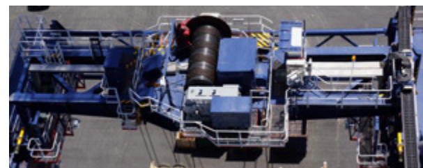
Picture 3.67: The second trolley on a modern STS crane.
