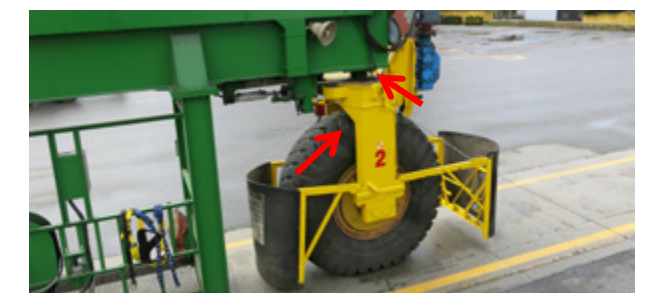
Picture 3.5: RMG crane driven at 5 of 6 wheels.
