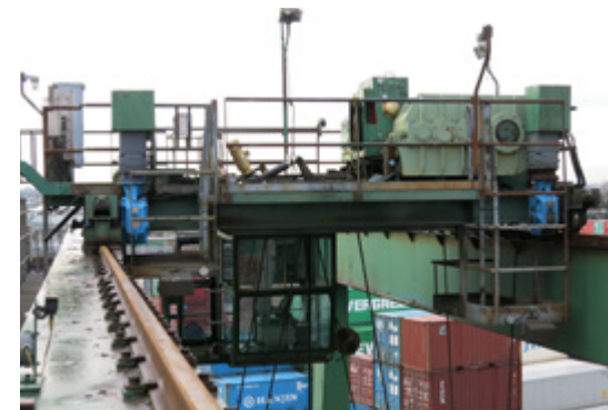
Picture 3.69: RTG trolley that is also suitable for ASCs.
