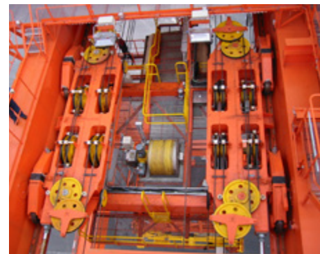
Picture 3.66: STS continuous rope support trolley.
