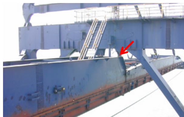
Picture 3.19: WS TGSB with pinned connection to plate girder boom.
