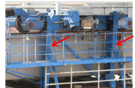
Picture 3.62: Main carrying members on trolley frame.
