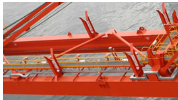
Picture 3.31: Twin girder boom with cross beams and diagonal bracing.
