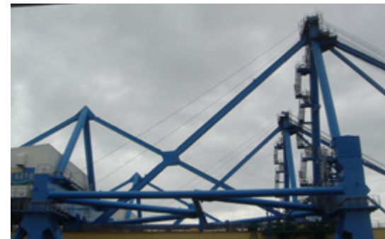
Picture 3.42: Crossing tension members, landside and waterside upper diagonals.
