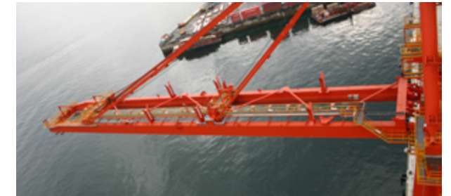
Picture 3.34: Twin girder boom with tie beam.
