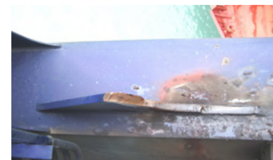
Picture 2.8: Looking down on a forestay connection plate that failed in fatigue.
