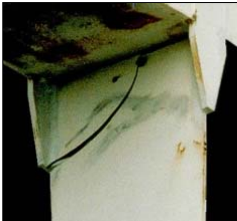
Fatigue Failure on Low Profile Crane Boom Hanger
