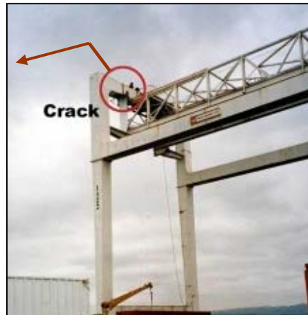
Fatigue Failure on Low Profile Crane Boom Hanger
