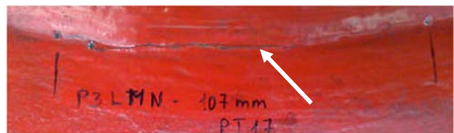
Intermediate equalizer beam crack (lower photo) that is obstructed by the pin ear plate in the upper photo.
