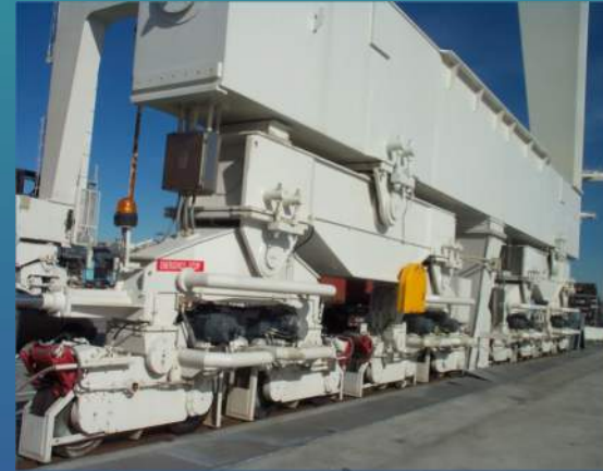
Gantry rotation to accommodate curve
