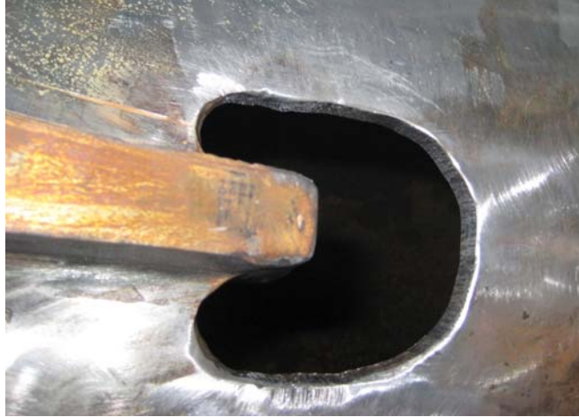
Figure 4: Stress relief hole at the end connection before grinding
