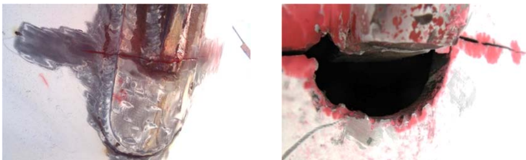
Figure 7: Cracking propagated from notches in pipe
