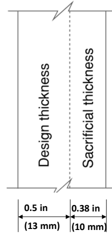
Sacrificial thickness (example below is based on side of float)
