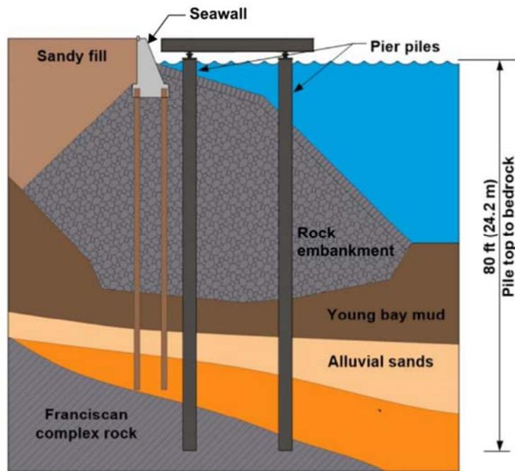
Figure 4. Elevation of pier and seawall.
