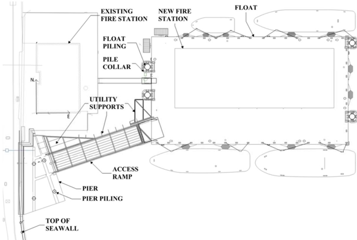
Figure 1. Plan view of facility.
