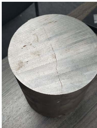
Figure 9. Cracked high-strength pin.
