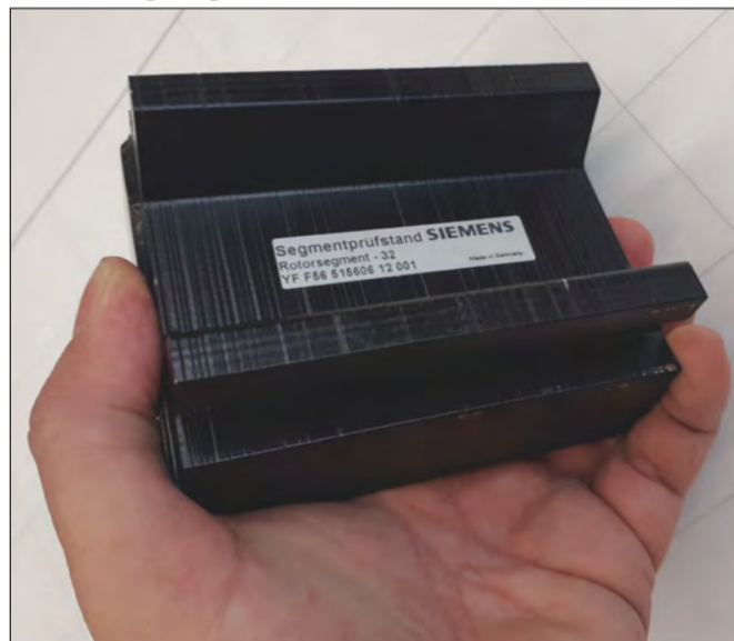
Permanent magnet segment as used in the test motor
