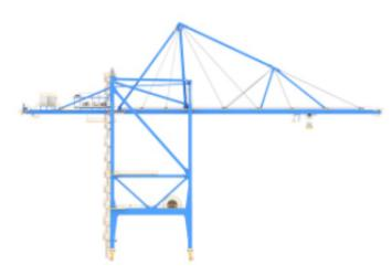
The Balance Crane is a concept Liftech unveiled in 2019 (WorldCargo News January 2019, P. 1). It features an elongated boom that extends back to the landside legs of the crane, with a shorter crane girder section that remains horizontal as it is lowered, as the boom rotates into the raised position for vessel clearance and stowage.
