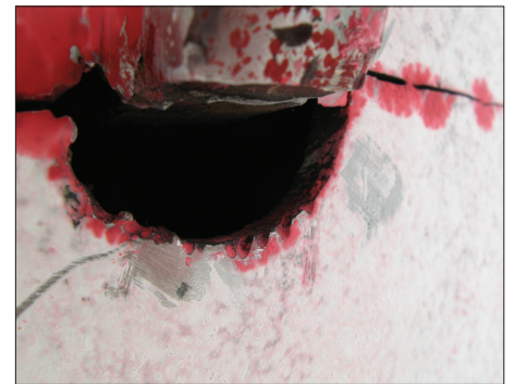
Figure 3: Roughly cut stress relief hole
