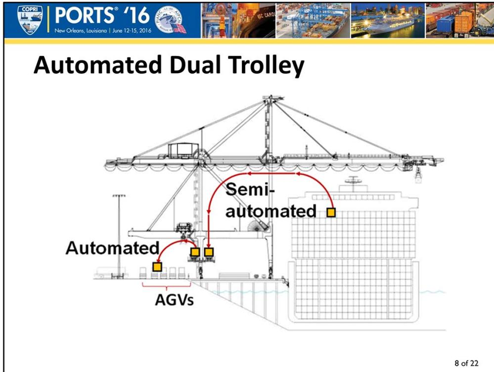
This shows the typical arrangement for automated terminals. It sometimes includes the option for a tandem 40' lift ship trolley.
