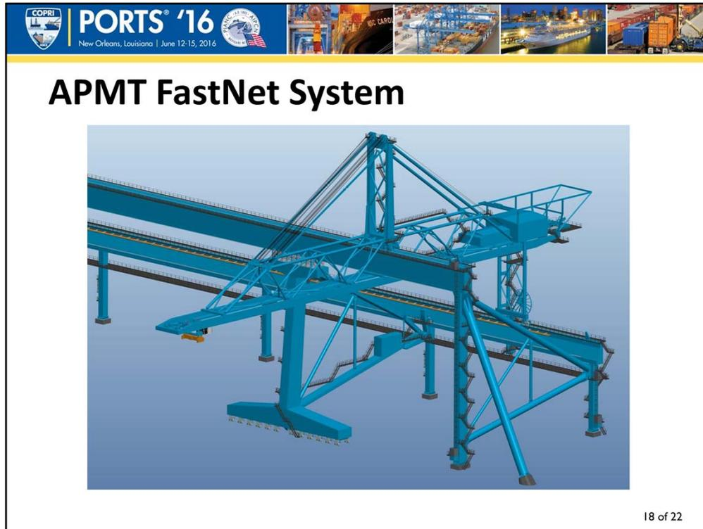
Fixed elevated girders are used at the landside to facilitate yard equipment access under the cranes.
