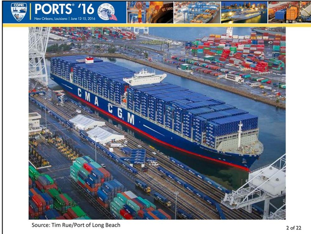
Container ship sizes now carry nearly 20,000 TEUs. However, most of this added capacity is due to increased container stacking heights and increased stack widths. Ships haven't gotten much longer, so the number of container cranes that can fit along the ship has increased little.
