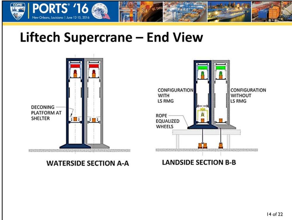
This system has separate rails for adjacent cranes, for nesting of gantry and improved stability.
