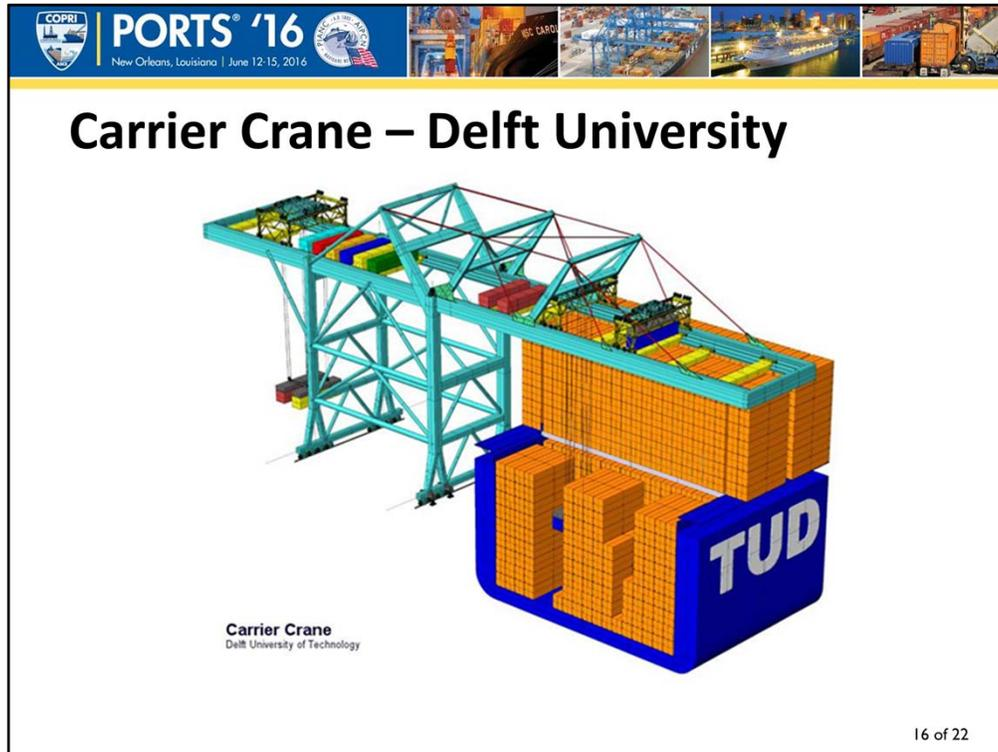
The Carrier Crane developed by Delft University includes multiple waterside hoists that lift containers onto carts which transport the containers to a landside hoist that services the yard equipment. The landside hoist handles two containers at a time.
