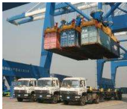
Figure 2. Dual hoist – triple spreader system.
