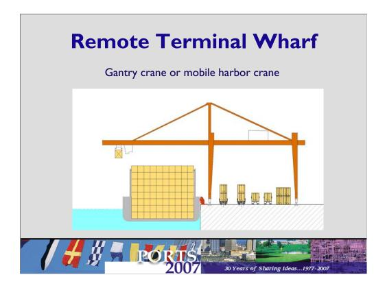
Containers can be loaded directly to rail if properly sorted, or the containers could be set on the inland wharf and the sorted using the gantry crane. A conventional Panamax crane or a harbor crane, such as a Gottwald, could handle containers.
