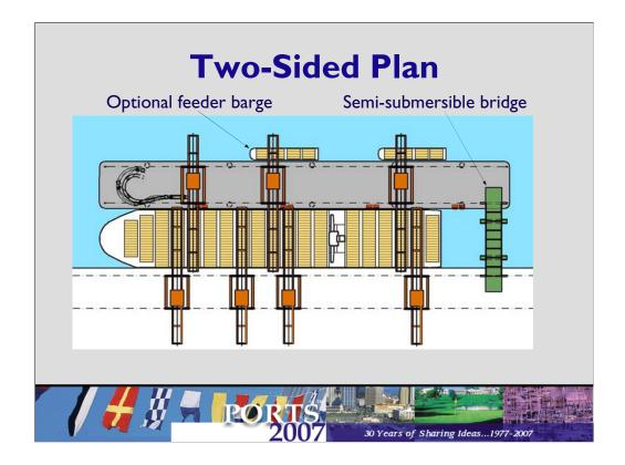
The ship is berthed between a marginal wharf and a movable offshore crane barge.
