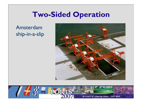
Now we'll discuss the secondary application, the two-sided operation. In this operation, a ship berths in a slip with cranes on both sides.
