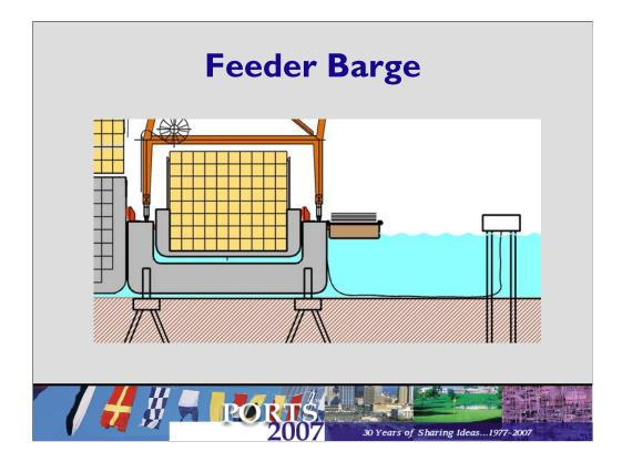
Recall the capacity of each feeder barge is 400 FEU. This means that for each barge traveling upstream, 400 fewer trucks are traveling on the road.
