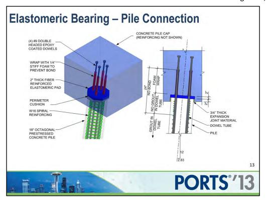
For the McNear's Beach Park Pier design, compared to the specimens tested at the University of Washington, the dowels are unbonded for two feet and a 2" thick pad is used instead of a  $\frac{3}{4}$ " thick pad.
