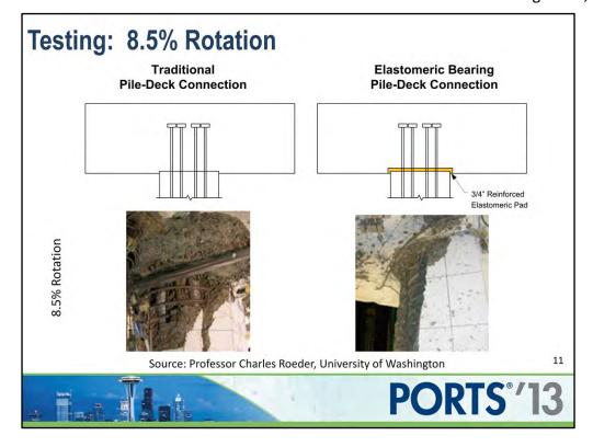
At 8.5% rotation, the concrete in the core of the Traditional Connection crushed and failed. The outer concrete shell of the Flexible Connection spalled but the core was intact. Local "buckling" deformation of the reinforcing dowels occurred near the pileto-cap boundary as the bars elongated in tension when the piles were rotated in one direction, and then compressed when rotated in the opposite direction.
