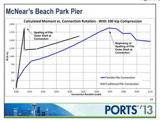
For the McNear's Beach Park Pier design, calculations based on specified yield and failure strains indicate that the outer shell of a Traditional Pile Connection design would spall at about 0.6% rotation and the McNear's Beach Park Pier Flexible Connection at 7% rotation. Failure of the Traditional Connection is estimated at about 5% rotation. Failure of the Flexible Connection is estimated at over 10% rotation.
