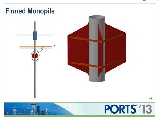
The idea is to add steel plate fins to a steel pipe pile to develop more soil reaction higher on the pile and reduce the bending moment and deflection.
