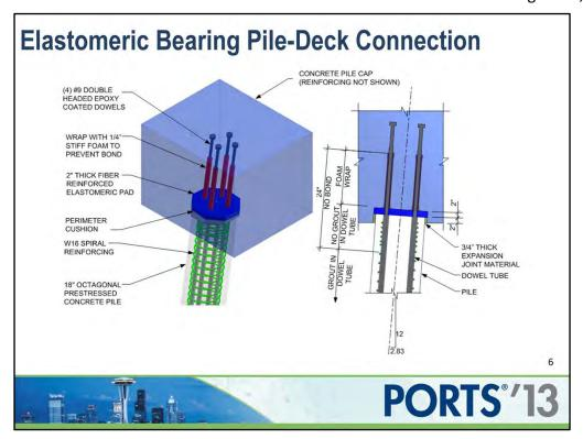
To meet the more stringent seismic criteria using the same pile design, a more flexible pile connection was developed. The flexible connection uses unbonded dowel lengths to allow the bars to stretch farther elastically, and a fiber reinforced elastomeric bearing to allow the end of the pile to displace in compression farther into the pile cap.
