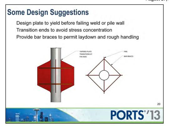
The geometry of the fin will depend on the soil properties.
