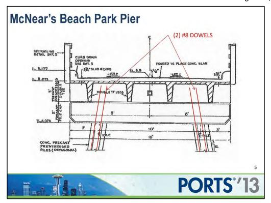
The repaired structure had to meet a more stringent design criteria than the original structure, and the number and size of the piling could not be increased due to permitting difficulties.
