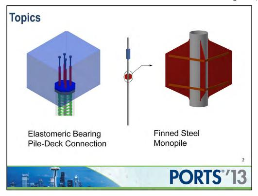
This presentation will cover two topics: a pile connection that uses an elastomeric bearing and unbonded dowel lengths to increase flexibility, and adding fins to steel piles to reduce bending.
