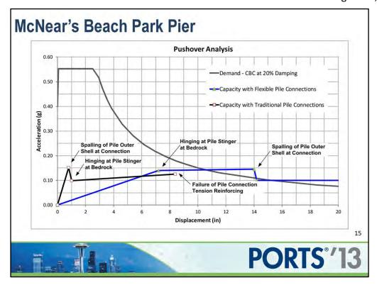
This graph presents the design displacement demand at an estimated 20% damping and the calculated lateral displacement of the structure for a design that uses a Traditional Pile Connection and a Flexible Pile Connection.
