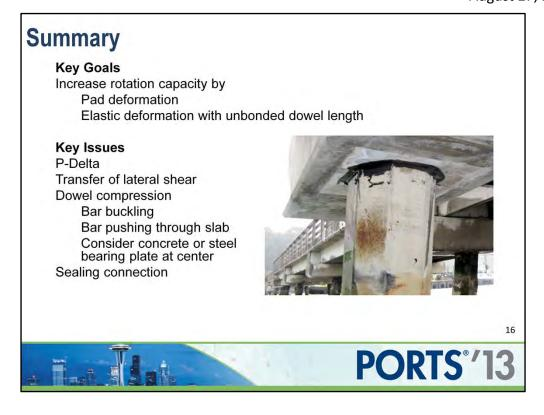
In summary, the key goal of the Flexible Pile Connection is to increase rotation capacity while maintaining connection strength. This goal is obtained using the elastomeric pad, perimeter cushion, and unbonding the dowels for some length.
