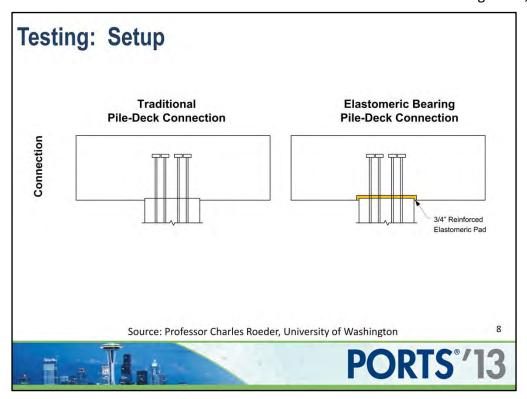
A variety of pile connections, including connections with elastomeric bearing pads, have been tested by Professor Charles Roeder of the University of Washington. The next slides present test results of two piles selected from many tests, one with and one without a bearing pad. These tests used 24" prestressed octagonal piles, a large 450 kip axial loading, and a  $\frac{3}{4}$ " thick reinforced elastomeric pad.
