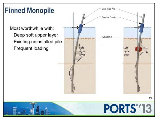
For a steel dolphin pile on a recent Liftech project, four large steel fins were added to significantly increase the soil resistance on the pile.
