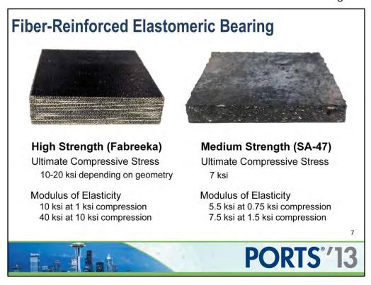
For the McNear's Beach Park Pier project, a high strength elastomeric pad was required. Less costly, lower strength, more flexible pads are also available.
