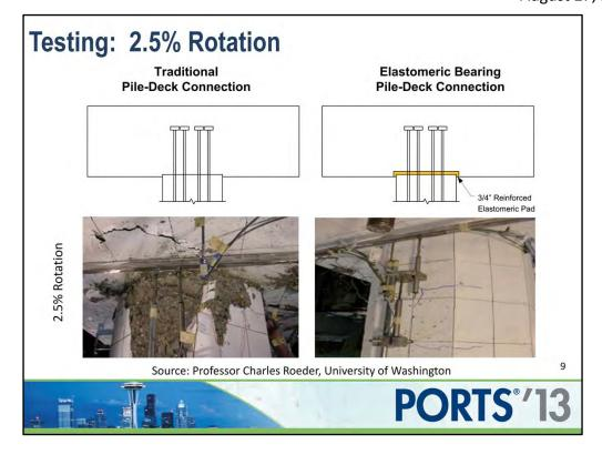
These photos are of test piles pushed laterally to obtain 2.5% rotation at the pile connection.
