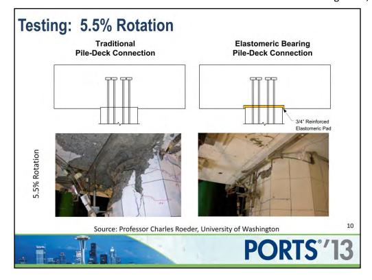
At 5.5% of rotation, the Traditional Pile Connection experienced severe spalling of the outer concrete shell, exposing multiple turns of the inner core spiral reinforcing. The Flexible Connection had more significant cracking, but no spalling.
