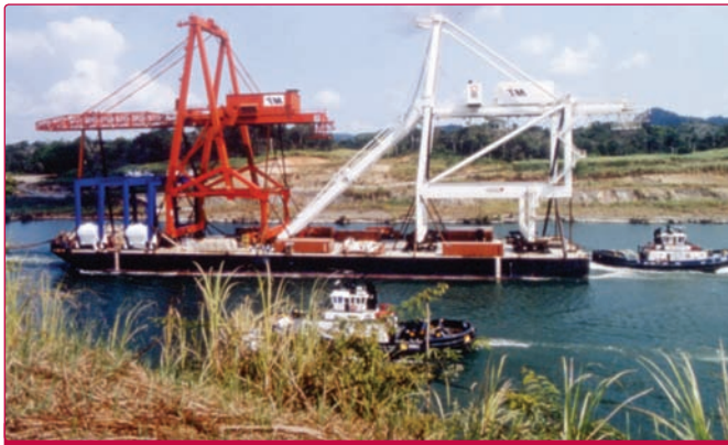
Figure 5. Relocation to another terminal by barge (note gage change modifications).
