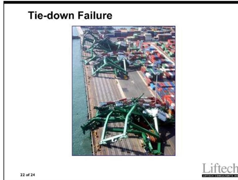
...and this type, which is often due to improper design of the crane-to-wharf tie-down connection.
