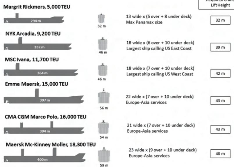
Figure 1: Important ship sizes currently in service
