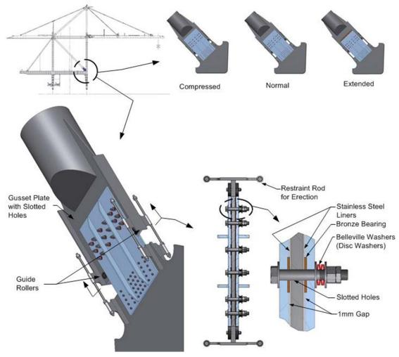
Liftech Seismic Damper
