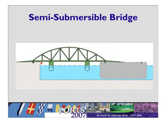
Pontoons lift the semi-submersible bridge so it can be easily moved to and from the operating position.
