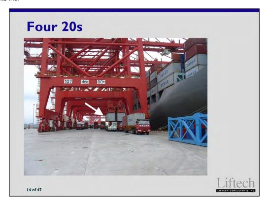
Two tractors and chassis have been positioned to receive the containers. Good drivers can position the two chassis as fast as one and still meet the geometric requirements of the crane.
