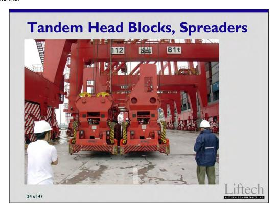
Each headblock is connected to its captive spreader in the usual way.
