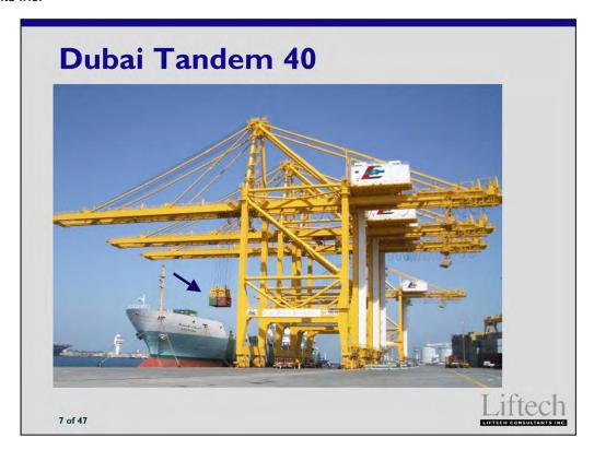
ZMPC has provided dual hoist tandem 40 cranes to the Port of Dubai. These cranes are conventional and do not have special IBC connection removal platforms or a shore hoist.
