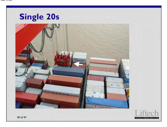
The crane can handle single 20s while both spreaders are attached, or the second spreader may be locked to the trolley in the idle position.
