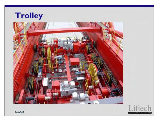
The trolley – a duplex of a single hoist rope trolley.
