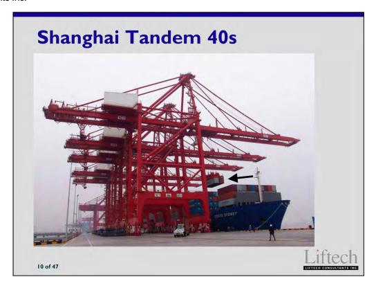
The ZPMC crane in Shanghai, China is the first tandem 40 dual hoist crane.
