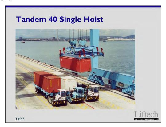
Some tandem containers are handled with one headblock and two spreaders. The single headblock tandem lift system has a significant disadvantage of needing to be balanced.
