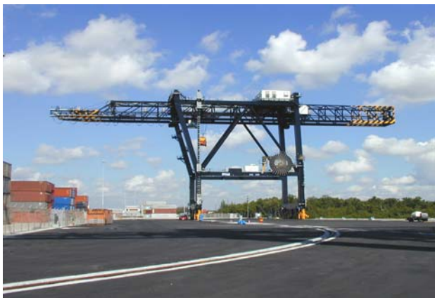
Figure 14: 16-Wide Low Profile Crane at Port Everglades
