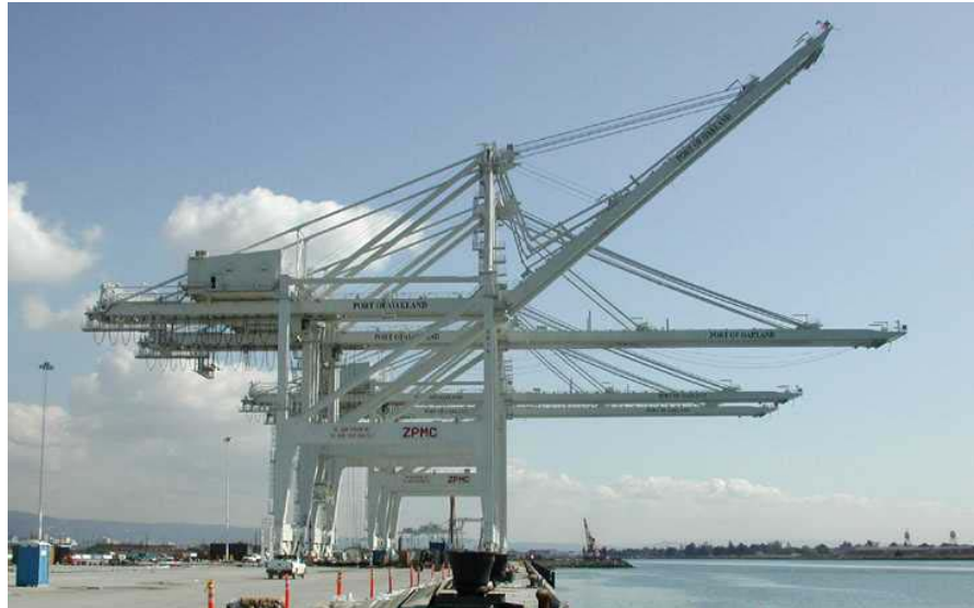
Photo 3: Port of Oakland Berth 57 Cranes, 213 Ft Outreach, 100 ton Cargo Beam, 2002
