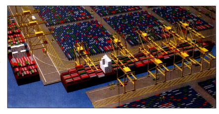
ship turn. The study was performed using the JWD/Liftech General Marine Terminal Simulation and the CraneSim computer models. Nine cranes can unload and load the ship in less than 15 hours.
