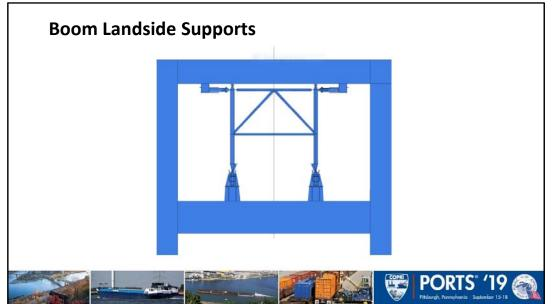
The boom support wheel positions are adjustable to compensate for construction tolerances. Preloaded equalized hold-down rollers are provided at the top, similar to at the waterside (not shown in the image). The preload keeps the wheels in contact with the boom upper rail, even when the boom is at the full backreach position.
