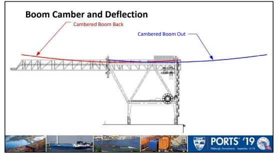
In the modern LPC, the boom deflection at the outreach with the trolley at the outreach is 30 in (760 mm).
