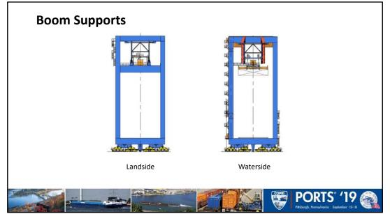
Specially shaped waterside hangers are used for smooth and structurally reliable boom travel. The special shape of the hanger eliminates lateral loads on the hanger. The side rollers that bear on the upper chord resist boom lateral loads. An equalized truck with two boom support wheels bear on the rail bar below the lower chord.
