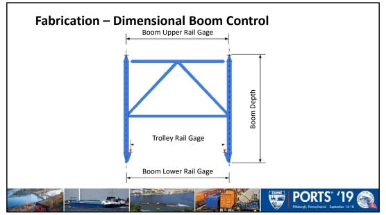
Fabricating a very large truss 120 m (400 ft) long is difficult, but a greater challenge is controlling the dimensions between the upper and lower chord rails, the out-to-out dimensions of the upper chords, and the dimensions between the trolley rail and the boom rails.
