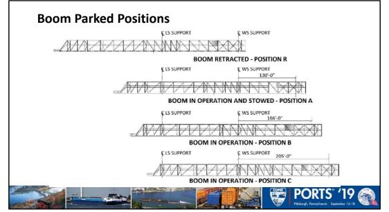
When the LPC is operating over a small ship, locating the boom at positions A or B reduces the boom reach from the face of the wharf and reduces boom positioning time. Position C is only used for operating over a large ship. During a hurricane, the boom is centered (position A), reducing the landside and waterside lateral wharf loads. Position R is necessary to allow the crane to clear a vessel during gantry travel and for normal stowage, when high winds are not forecasted.
