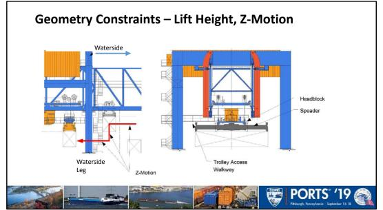
"Z-motion" maximizes the lift height. The trolley is designed such that the headblock and spreader (lift system) nest high into the trolley, gaining about 1 m (3 ft) of lift height, for removing the top row of containers, depending on the vessel and tide level. However, the lift system must be lowered to clear the waterside hangers, just waterside of the vessel.
