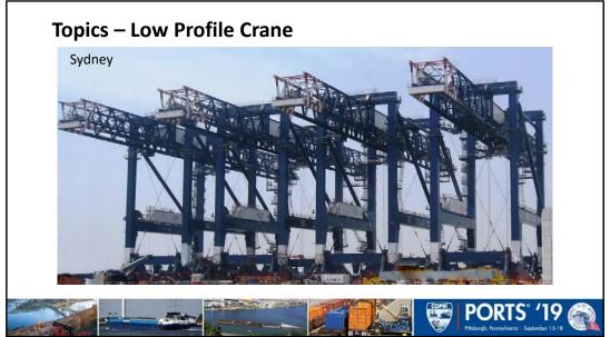
Numerous container terminals have significant height restrictions caused by proximity to airports. Low profile ship-to-shore container cranes (LPCs) are vital to these terminals. LPCs servicing ultra-large container vessels are significantly heavier and more complex than conventional A-frame cranes (AFCs), and present a myriad of new challenges for crane and wharf designers.
