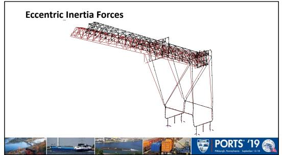
When traveling along the wharf, with the boom out or retracted, eccentric inertia lateral and vertical forces tend to twist the crane, with calculated maximum of 1 m (3 ft) deflection (deflections shown are not to scale).
