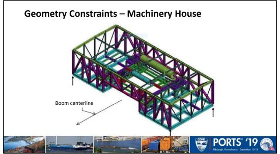
The highest point of the crane is the roof of the machinery house for the main hoist and boom shuttling—minimizing height is important. The house straddles the boom and includes a higher-elevation center deck above the boom and two lower-elevation side decks. The multi-level deck needs trusses to keep it integral. Because the main hoist drum straddles the left and right decks, the frame size and stiffness is sized with consideration to keep the couplings from failing.
