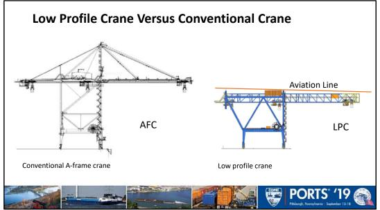
Note that the conventional A-frame crane (AFC) is much larger than the low profile crane (LPC).
