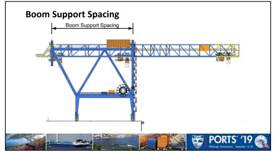
Spacing affects reactions, which affect the boom supports, and boom and frame structure and weight. Inclining landside legs increases boom support spacing, reducing the reaction and reducing the crane weight.
