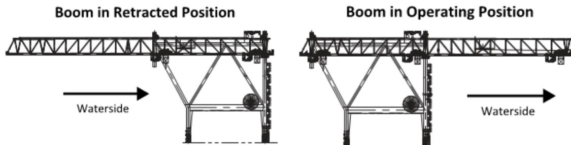
Figure 2. Low profile crane boom positions
