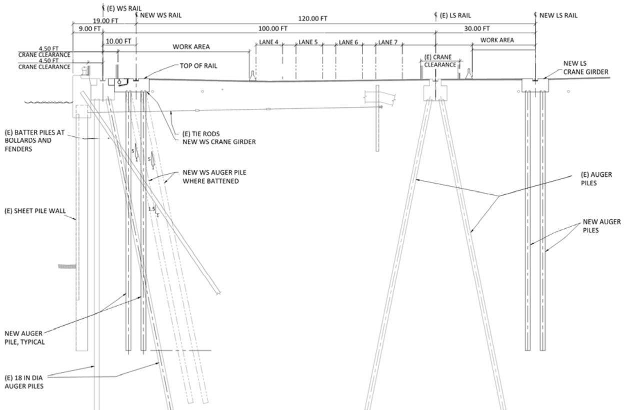
**Figure 5. Modified wharf section**
