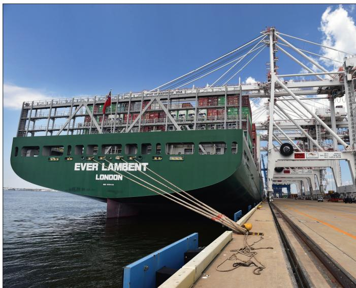
Figure 5: Suboptimal mooring line arrangements - all lines to one bollard
