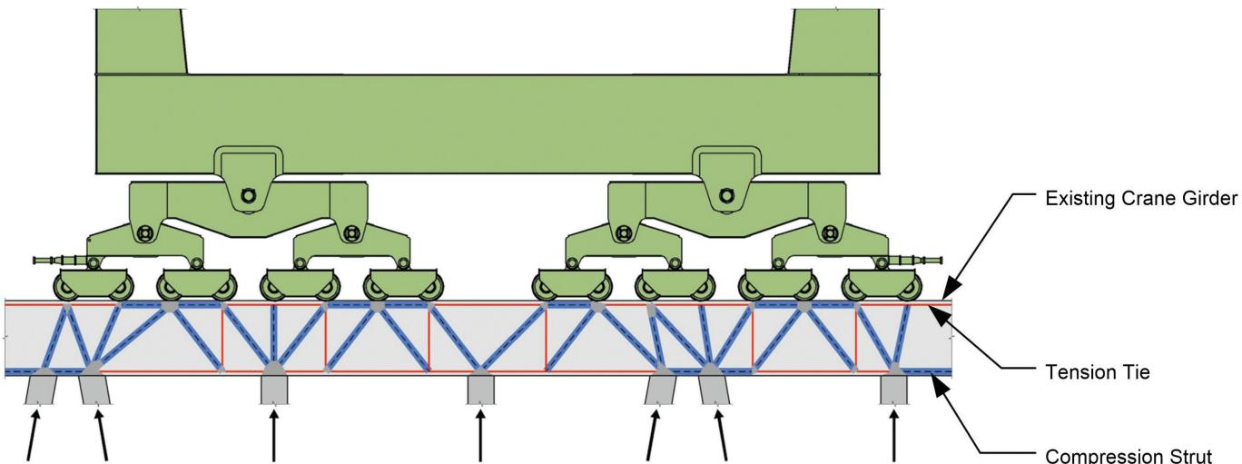
Figure 6: Strut-and-tie girder analysis
