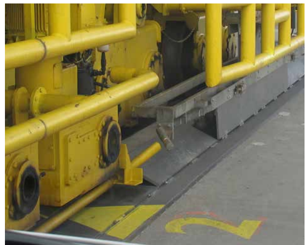
Photograph S: The pick-up system on STS crane powered by underground bus bar
