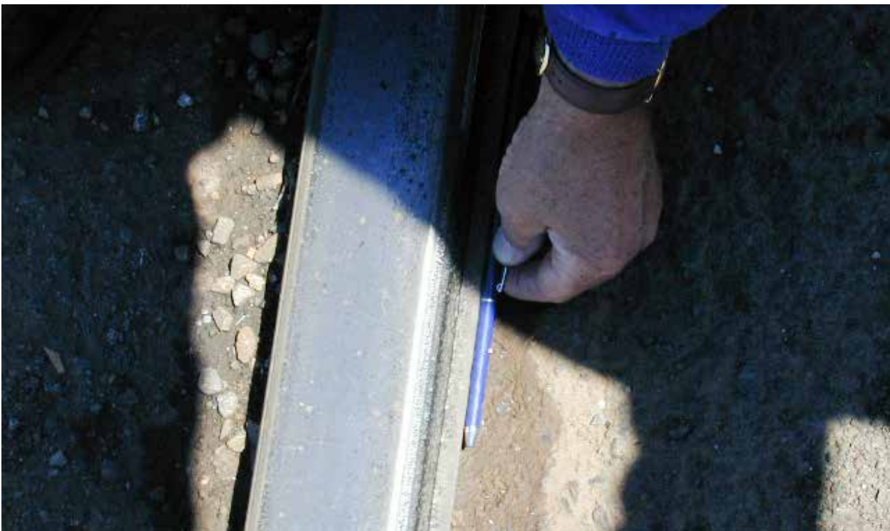
Photograph K: RMG crane rail worn from the side by wheels, likely due to crane racking while driving
