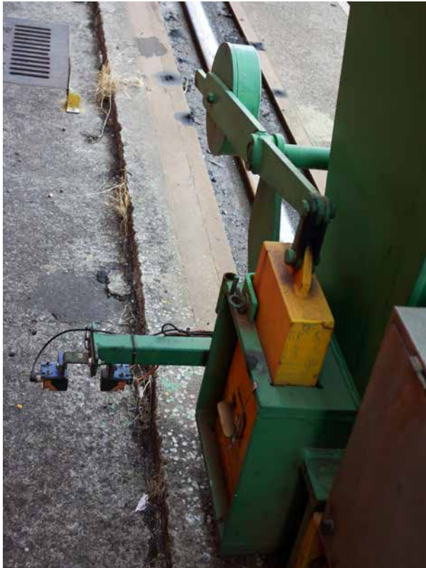
Photograph W: RMG positioning reader gate and flag in the background. Stowage pin in foreground
