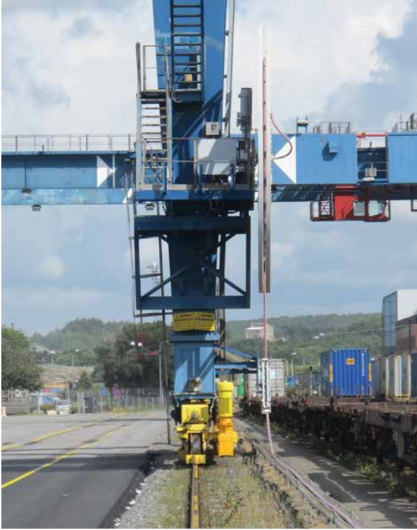
Photograph T: Standard cable reel solution on RMG
