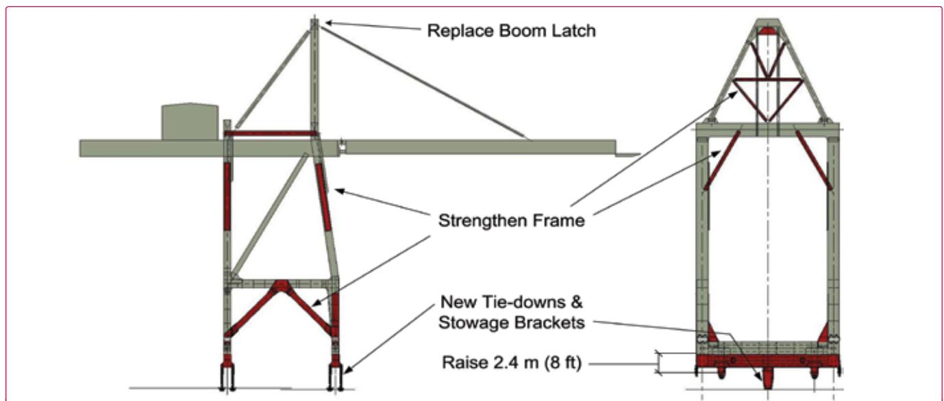
Figure 1. Structural modifications to accommodate larger vessels, new terminal requirements, and adjustments to a new terminal due to relocation.
