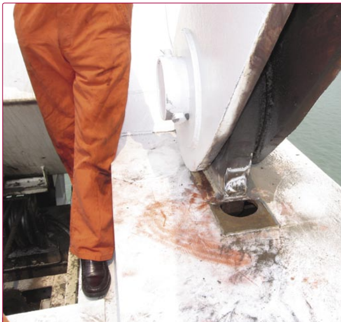
Figure 4. Relief hole at inner forestay-boom connection.
