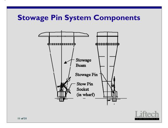
Socket depth sufficient for strength and for non-hurricane corner uplift
