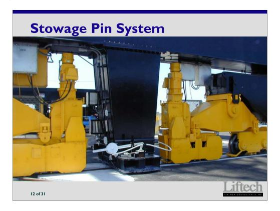
The lever mechanism links the pins on each side of sill beam so both pins can be raised or lowered at the same time.
