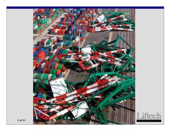
We have not experienced a case where a collapse has resulted from the crane structure failing prior to a stowage system failure.
