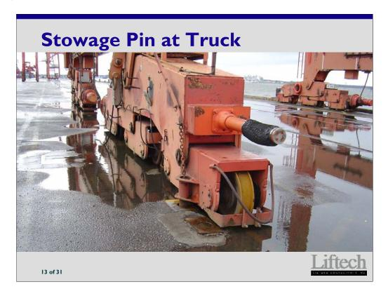
This photo shows the stowage pin on truck. Because the stowage pin is only on one corner per side and only one side per rail, this torques the truck.
