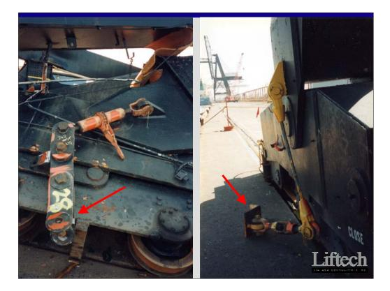
On the left, tie-down link plates separated and released from the pin. (See the next slide for a schematic of a similar failure mode at the wharf bracket.)
