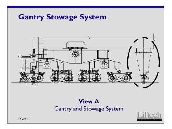
Stow pins at the center of the sill beam to prevent **leveraging** effects in the gantry system.
