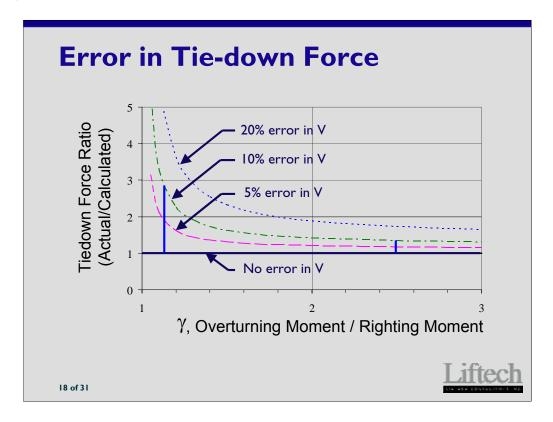
As the ratio of moments increases (bigger uplift), the error in the calculated tiedown force approaches the error in the wind force.
