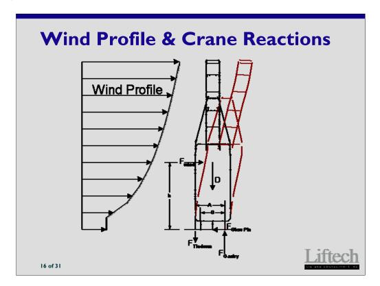
Proper load paths are required for loads in all directions.
