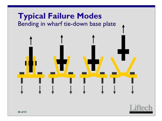
Improperly designed base plate. The base plate bends, allowing the bracket to open up, releasing the tie-down.
