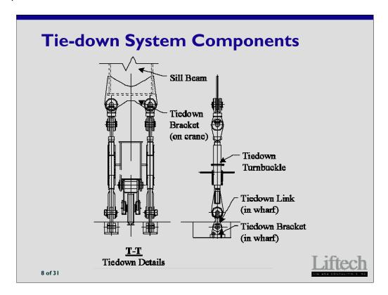
Designed for rotation and displacement of the sill beam. Split calculated design load 60/40 due to unequal load sharing.
